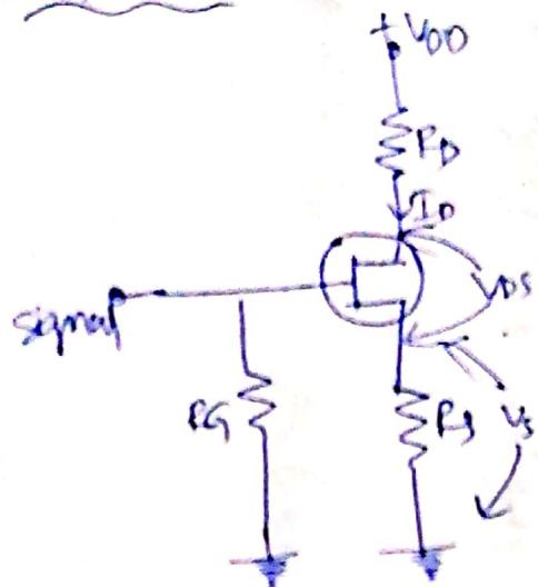
$$V_S = I_D R_S = I_S R_S$$
